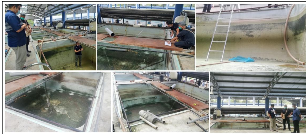
Figure 19. The Simulation Tank for Simulation Light and Moving Images on Top Water Lure (15ft L X 15ft W X 12ft D)
