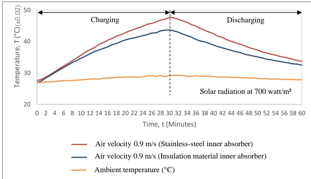
Figure 3. Outlet Temperature Histories Between Stainless Steel Inner Absorber and Insulation Material Inner Absorber for Pre-Heating Experiment
