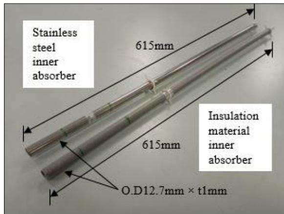
Figure 2. d The Insulation Material and Stainless-Steel Inner Absorber Without Perforated Fin
